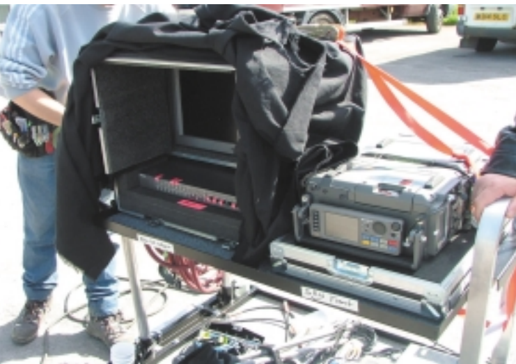
Hardware set-up: HDCAM SR deck with 17-inch HD monitor for raw log output — which can be switched to give a colour-corrected video look
