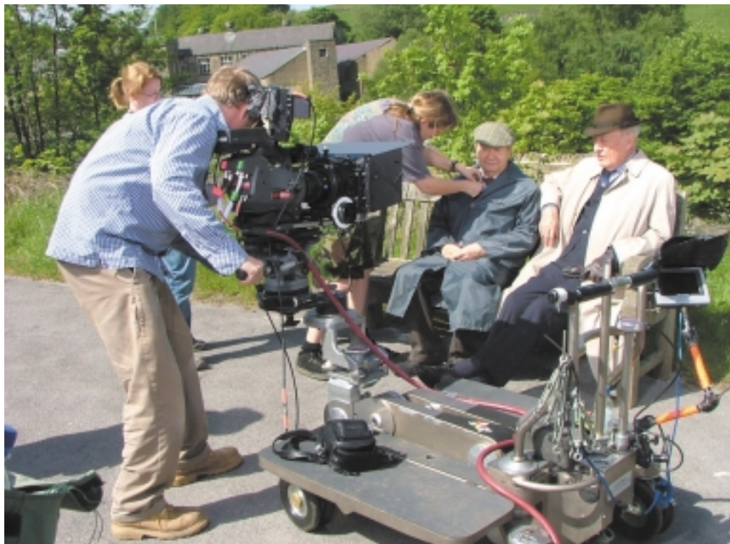
The Viper captures raw 4:2:2 files at 1080P 25fps to a Sony SRW1 HDCAM SR deck using a set of six Zeiss Digi Primes
